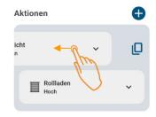
You can change the sequence of actions by holding down the action and then dragging it to a different position.
