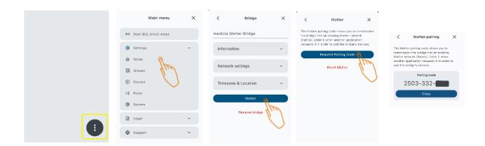
Open the settings and select your *Home*. Click on your mediola Matter Bridge to open the bridge settings. Click on the *Matter* button and then the *Request Pairing Code* button to generate a pairing code. Copy your pairing code and open the respective app.
