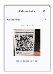
Then put the device in teach-in mode. Now click on *Next* to teach the device to the bridge and integrate it into the mediola Connect app.
